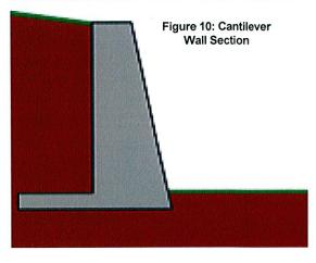
levered base is reinforced and is designed to prevent uplifting at the heel of the base, making the wall strong and stable. Reinforced concrete cantilevered walls sometimes have a batter. They can be faced with stone, brick, or simulated veneers. Their front faces can also be surfaced with a variety of textures. Reinforced concrete cantilevered walls are typically poured in place using forms. When the use of forms is not desired, reinforced concrete block cantilevered walls are an option.
